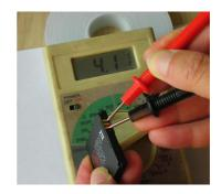
Please note the voltage doesn't indicate how much remaining capacity of the battery has. You need to check that with oscilloscope connected (see below).
