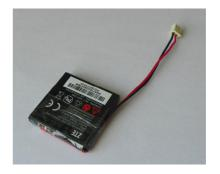
The battery is to be attached to the inner side of back cover (for 094) or back plate (for 096) with double-sided adhesive foam. This adhesive foam is included in purchase and has been put in place before shipment. You need first determine battery position and orientation so as the connecting wire is run smoothly (see photos below as examples). Then peel off the protection paper on foam and press battery firmly on to it.
